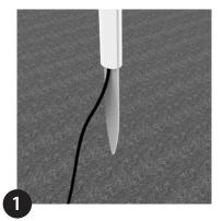
Locate a suitable exterior location with semi-soft ground (Grass or soil) and push spike firmly into position, using level to ensure vertical alignment.
